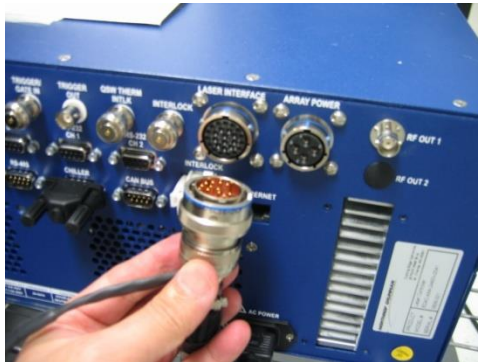
Figure 4-10 Laser Signal Cable
