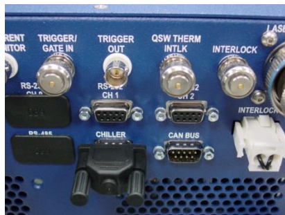
Figure 4-15 BNC Interlock Connection
