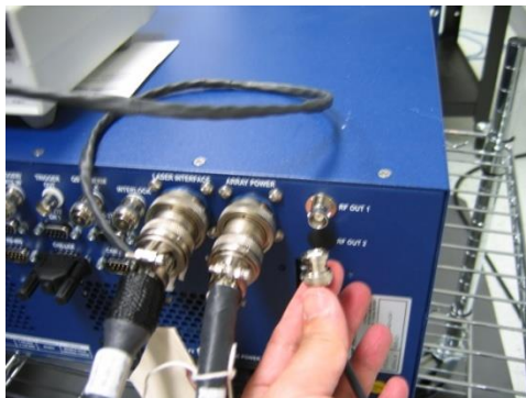
Figure 4-12 RF Signal Cables
