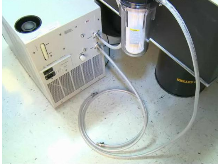
Figure 4-4. Chiller Assembled with Coolant Hoses and Filter
